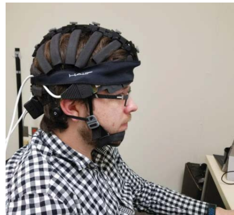
Figure 2. Setup of simultaneous fNIRS and EEG headgear
