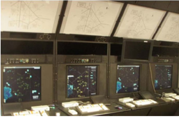
Fig. 3. Air traffic controller's simulation center: Each workstation consisted of a high-resolution ( 2048 \times 2048 ), radarscope, keyboard, trackball, and direct access keypad.
