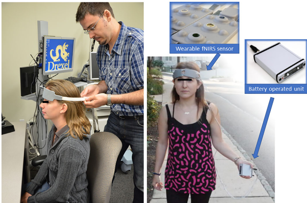
Figure 1 Wearable and miniaturized fNIRS sensors allow for the monitoring of brain activity in increasingly realistic and natural environments from minimally restricted office settings (left) to unrestricted outdoor settings (right).
